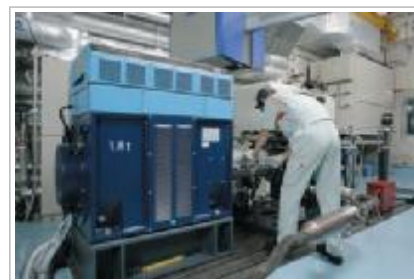
Oil pump test on engine dynamometer
