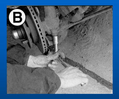
Loosen the strut lower knuckle fixing bolts and nuts.
