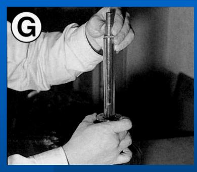
Make sure that lock ring has been securely tightened by hand. Please do not over-tighten! Please do not hit a piston rod of the cartridge by hand or tooling during the process of assembling.
